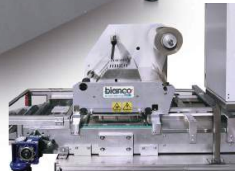
NSKT automatic sealing machine: reel detail.
